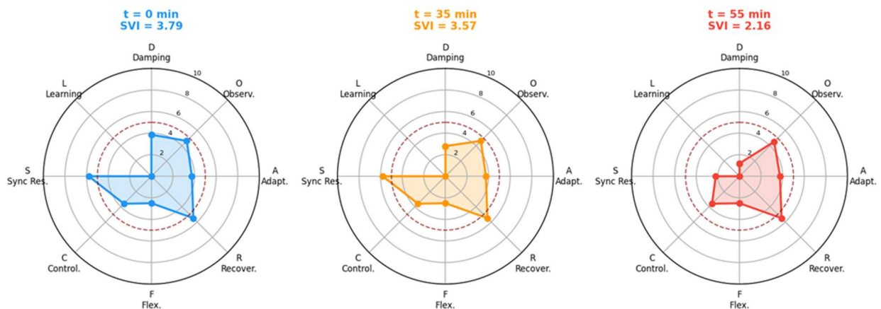
Figure C-1. SVI dimension radar at t = 0, 35 , and 55 min. The red dashed circle marks a uniform per-dimension value equating to SVI_{final}= 5.0 . Collapse of D (Damping) and S (Sync Resistance) drives most deterioration.
