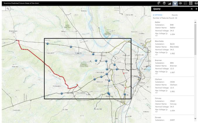
Fig.7 View stations with voltages above or below user-defined threshold
