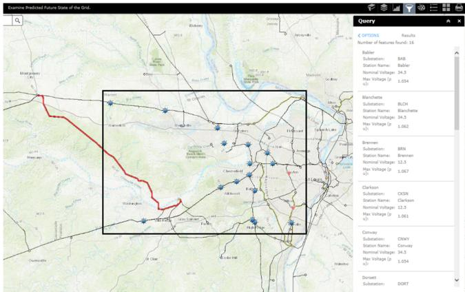
Fig.7 View stations with voltages above or below user-defined threshold
